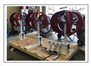
per multi-turbine tower. In addition to increased capacity for electricity generation, other benefits related to this integrated turbine technology include ground level installation and maintenance of fewer generators and electrical components, options to reduce noise, and lower transportation barriers and costs.
